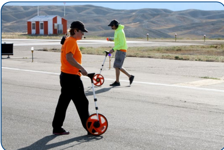
Aviation Planners Kaitlyn Westendorf (left) and Todd Green (right) perform Pavement Condition Index (PCI) Inspections.
